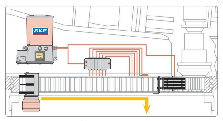
There is a gear wheel with two foam rubber plates on one axle. The intermeshing of the gear wheel and the toothed wheel causes the plates to move simultaneously. These wipes over the toothed wheel continuously remove any excess lubricant from the front sides. The foam rubber plates go through a stripper from where the lubricant is taken to the container that has to be emptied regularly.
